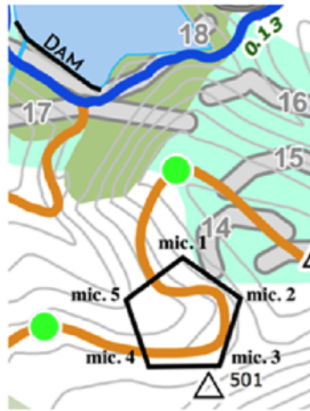
Figure 2. Map of Walnut Creek Park microphone setup location (each side of the pentagon is 30 meters), and corresponding concert loudspeaker configuration.
